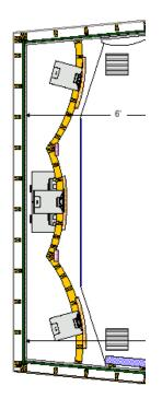
Figures 4 and 5: A curved speaker baffle wall
